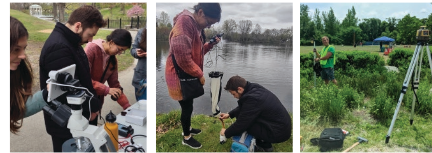
Volunteers use a fluorometer and microscope to examine and measure cyanobacteria. A plankton net is used by volunteers to collect water quality samples. Audubon Stormwater Manager Ryan Kopp conducts an elevation survey within existing green infrastructure.
